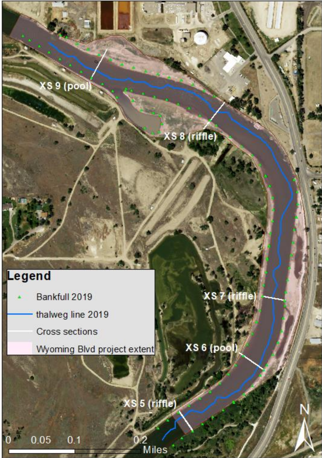
FIGURE 7. Bankfull elevations along the Wyoming Blvd project reach.
